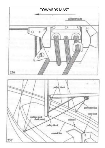
If the mainsail is taken aback, because of a windshift or the stern of the boat being kicked sideways by a following sea, BOOMLOCK TWO will prevent the boom swinging over. There is normally enough time for the helmsman to correct the course, so that the sail fills again on the original tack.
