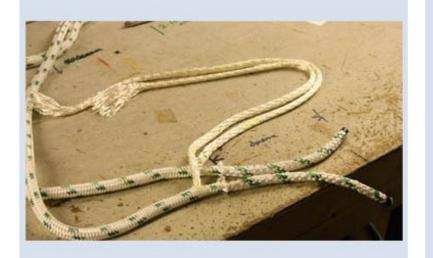
Repeat for the other end of rope and you will end up as this picture shows; with rope tails tapered
