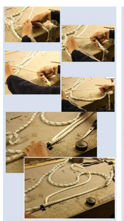
Grip at extraction point and pull bunched core over the tail to close up
