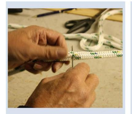
Thread a whipping needle with 120mm of fine whipping twine and double up, push through at intersection of splice. Pull through to leave two inch tail, pass needle through four times back and forth through rope. All stitches must be within the distance of 5mm
