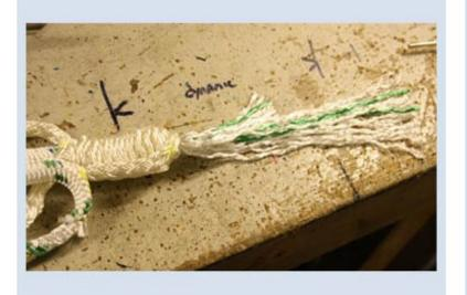
First of the three equal parts is to be cut at the grip point
