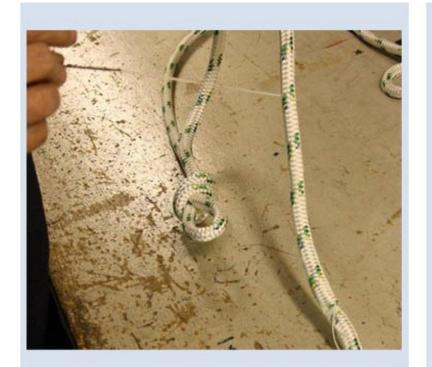
Continue passing needle back and forth through rope climbing about 30mm with each stitch about 200mm from splice cut whipping twine. Also trim off excess twine at splice
