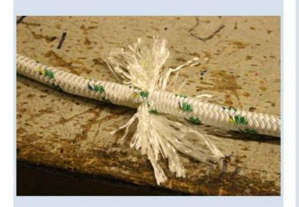
Pull hard from stopper knott to set splice at tightly as possible
