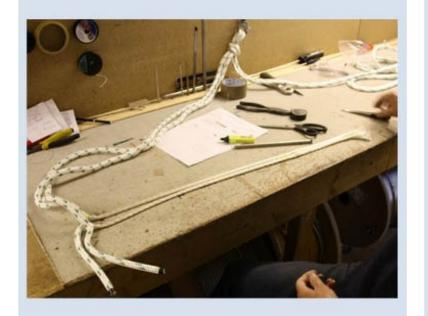
Pull the inner cores out
