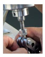
7- Ensure that the large plastic washer is seated on the top of the drum unit.
